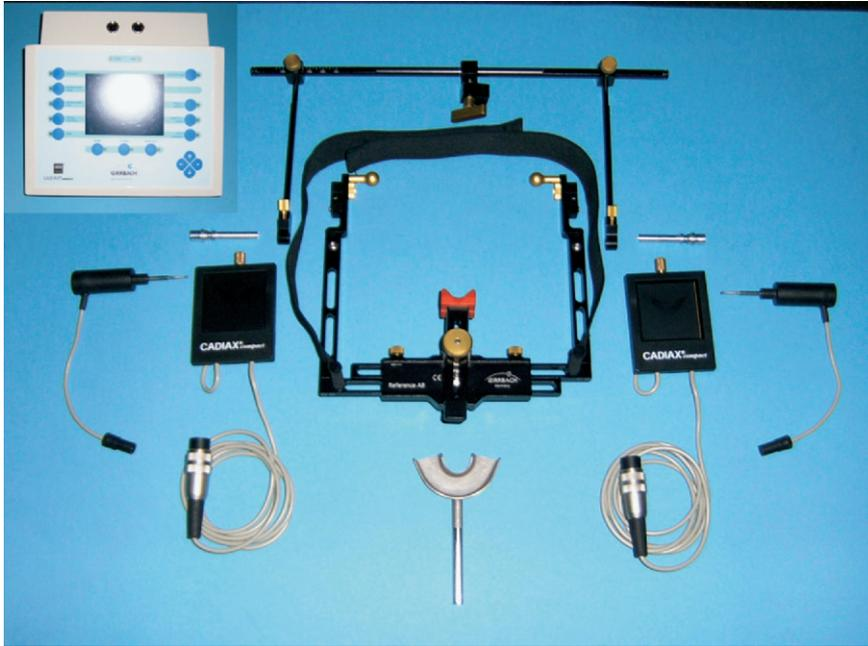
**FIGURE 1.** Overview of all components of the Cadiax compact system (electronic box is reduced in size).
